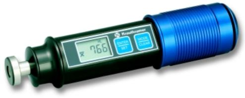
You can directly read the measured hardness value on the large LCD display. At the same time, the selected hardness scale (in this case HL) and the option Average  $\overline{\mathbf{x}}$  is displayed. The battery icon informs you about the current battery charge condition.
